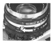
The KONICA S is provided with a built-in self-timer. With the M-X adjustment at position X, move self-timer lever to position V. The delayed shutter action device is now set, so the shutter will operate about 10 seconds after the shutter button is pressed.
