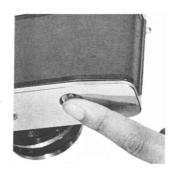
[2] Erect rewind crank and turn clockwise (in direction of arrow mark) to wind film into safety cartridge.
