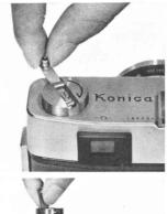
(3) When exposed film has been taken up into the safety cartridge, open backlid, pull out the rewindcrank spindle, and remove the cartridge. As the rewind operation progresses, the crank will tend to increase.
