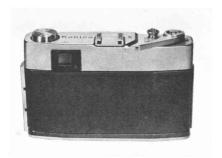
© Operate cocking lever and press shutter button. Repeat this action to bring start mark (black dot) of the exposure counter in alignment with the index mark.
